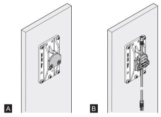
Fig. 12: Holder set, non-electrified (A) and electrified (B)
