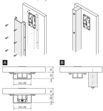
Fig. 7: Back panel reinforcement
