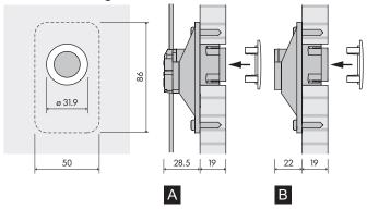
Fig. 19: Mono 20 P/L light with power cable (A) / non-electrified (B)
