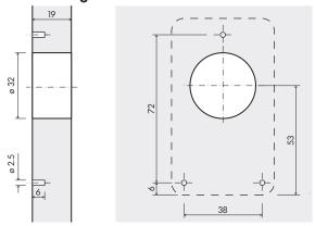
Fig. 21: Milled form for Mono 20 P/L light with cover clip
