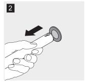
Fig. 15: Removing merchandise support
