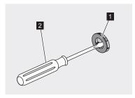
Fig. 17: Levering off cover clip
