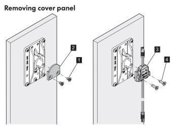
Fig. 13: Unscrewing cover panel
