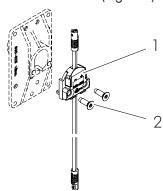
Fig. 4: Electrical connection set for non-electrified holder sets
