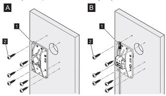
Fig. 10: Mounting on wooden panel
