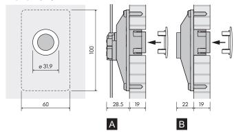
Fig. 18: Mono 20 P/L with power cable (A) / non-electrified (B)
